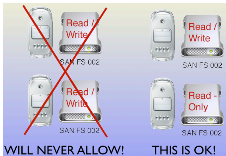
SERVERLESS SAN — SINGLE WRITER TO A FILE SYSTEM AT A TIME
